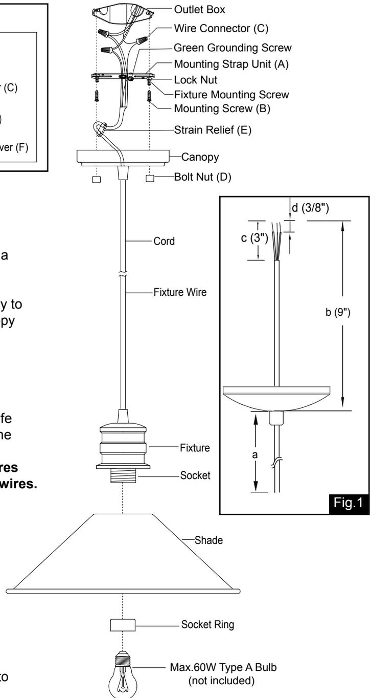
8. Pull the cord down slightly until the strain relief (E) touches the hex nut. Attach the canopy to the mounting strap unit (A) by inserting two fixture mounting screws, then secure it with two bolt nuts (D).
